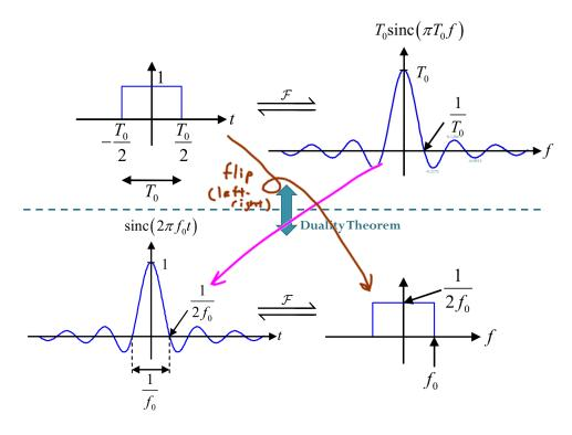
Figure 6: Duality theorem: rectangular and sinc functions
